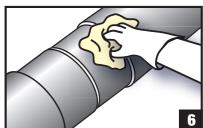
Air blast the steel and pipe coating to remove foreign contaminants. Surface must be clean and dry prior to application of product.
