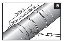
Ensure the pipe is at least 3°c above the Dew point before blasting to a minimum of near white to Class 2.5 with minimum 75 micron profile, peak to valley. Abrade at least 100mm of the line coating on each side of cutback area. For 3LPE coated Pipelines, use of a LPG gas torch to warm up the PE adjacent to the cutback area will ensure PE coating is dry.
