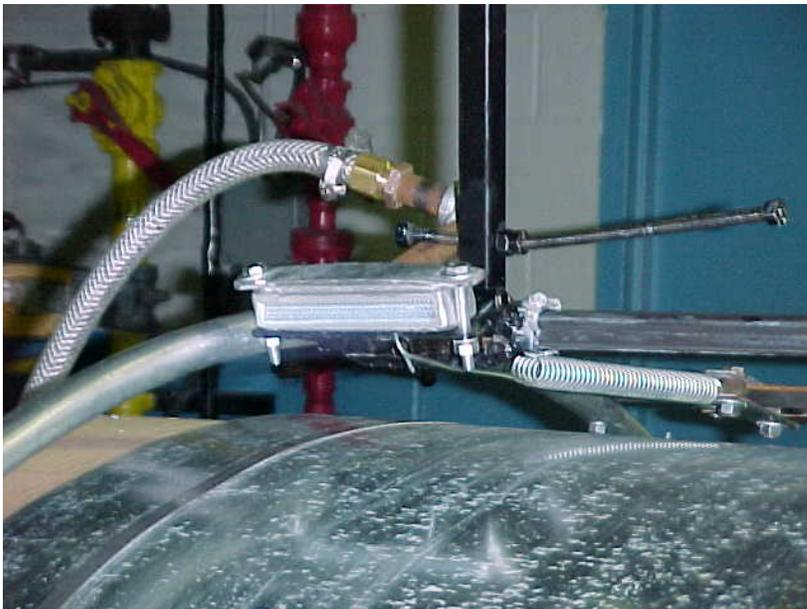
Fig 1 Burner used for Flame Treatment
